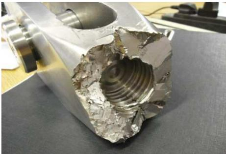
*Figure 3 Failed connector (not associated with the structures shown in Figures 1 and 2 or taken from a CROSS report)*
