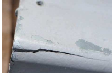
Longitudinal split (reproduced with permission)
