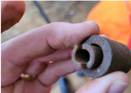
Figure 3: anchoring cylinder with two split wedges
