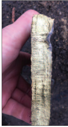
Steel section severed by linear cutting charge.
